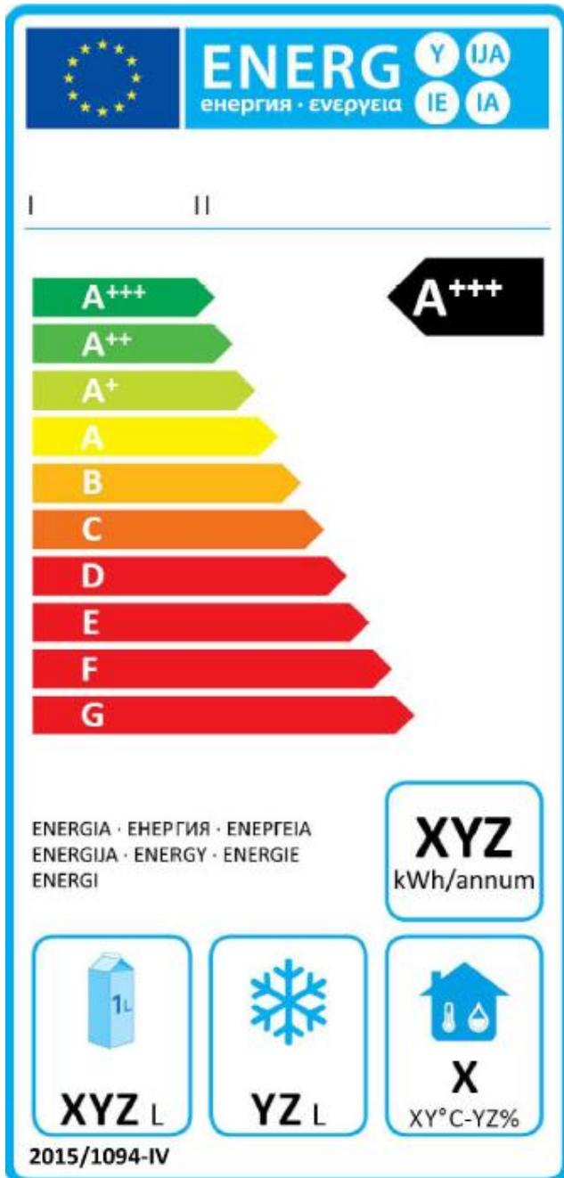
Figure1: Energy label for professional refrigerated storage cabinets
